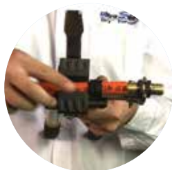
Set the fitting and the pipe in the tool
