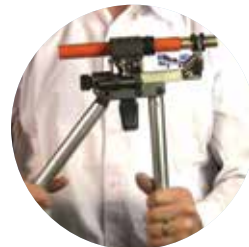
Connect the fitting and the sleeve to the pipe - in a single step
